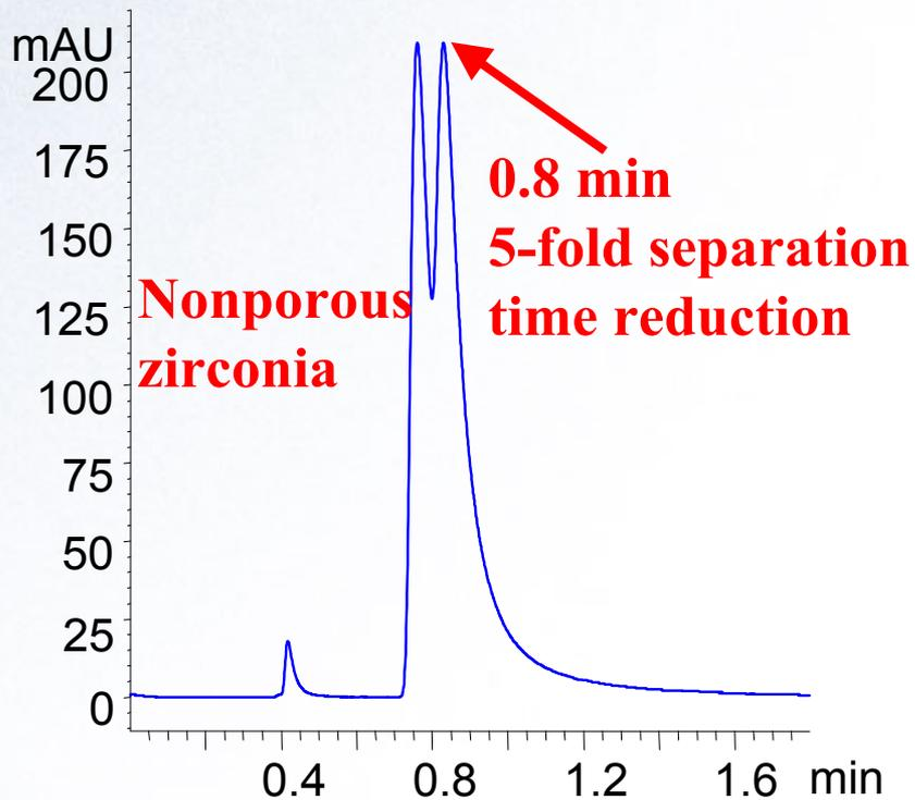
Chiral compounds on nonporous and porous zirconia-based DNB-L-PG anchored with APPA. Chromatographic conditions: mobile phase 99/1Hexane/IPA, probe solute: ( $\pm$ )trifluoroanthryl ethanol.
