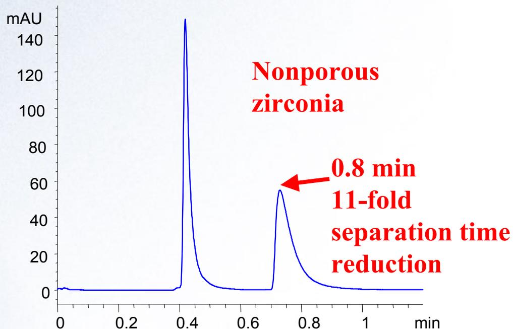
Chiral compounds on nonporous and porous zirconia-based DNB-L-Leu anchored with APPA. Chromatographic conditions: mobile phase 99/1 Hexane/IPA, probe solute: ( $\pm$ )1-naphthyl leucine ester.
