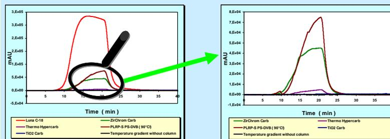
**Figure 2:** Signal intensity due to temperature programming for five different HPLC columns. Magnification on the right side does not include Luna C-18 column. **Detector: UVD at 254 nm**; flow rate of mobile phase (pure water): 0.5 mL/min; Temperature programme: 5 minutes at 30 °C, from 5 to 10 minutes from 30 °C to 200 °C, 10 minutes constant at 200 °C, then cooling down to 30 °C.
