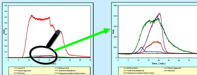
**Figure 3:** Signal intensity due to temperature programming for five different HPLC columns. Magnification on the right side does not include Luna C-18 column. **Detector: CAD**; flow rate of mobile phase (pure water): 0.5 mL/min; Temperature programme: 5 minutes at 30 °C, from 5 to 10 minutes from 30 °C to 200 °C, 10 minutes constant at 200 °C, then cooling down to 30 °C.
