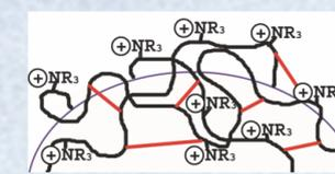
ZirChrom®-SAX is a zirconia particle coated with polyethyleneimine polymer and then crosslinked using a hydrophobic crosslinker. The crosslinker modifies the phase with a bit of reversed phase character, giving the ZirChrom-SAX phase a unique, multimodal selectivity.
