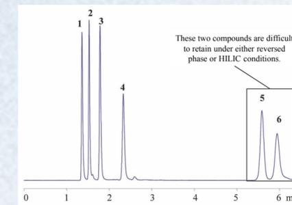
1=Thiamine (Vit. B<sub>1</sub>), 2=Pyridoxine (Vit. B<sub>6</sub>), 3=Nicotinamide (form of Vit. B<sub>3</sub>), 4=Riboflavin (Vit. B<sub>2</sub>), 5=Nicotinic acid (form of Vit. B<sub>3</sub>), 6=Ascorbic acid (Vit. C)
