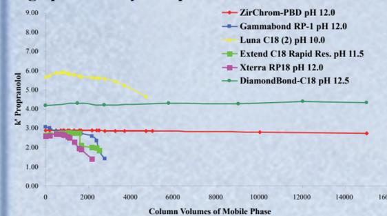
**Exposure Conditions:** Mobile phase, ACN/50 mM Potassium phosphate buffer at indicated pH; Temperature, 30 °C.
