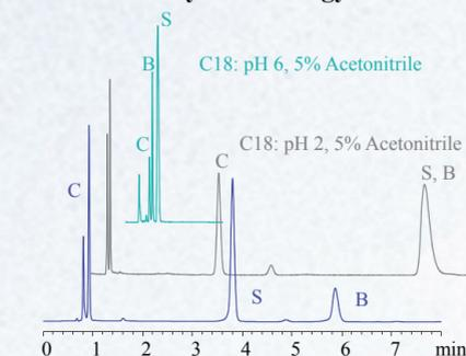
Columns: Leading C18 column, ZirChrom®-SAX, 100 x 4.6 mm i.d., 3 µm
