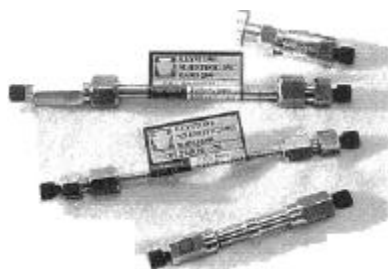
The Aquasil ® HPLC column from Keystone Scientific is now offered in a 3 \mu\text{m} particle size. Designed for highly aqueous mobile phases, the column is deactivated yet will not lose retention, even in 100% \text{H}_2\text{O} . The
