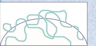
ZirChrom®-PBD is a zirconia particle coated with polybutadiene polymer and then crosslinked. The unique surface chemistry coupled with the polymer coating enables a superior, multi-modal selectivity.
